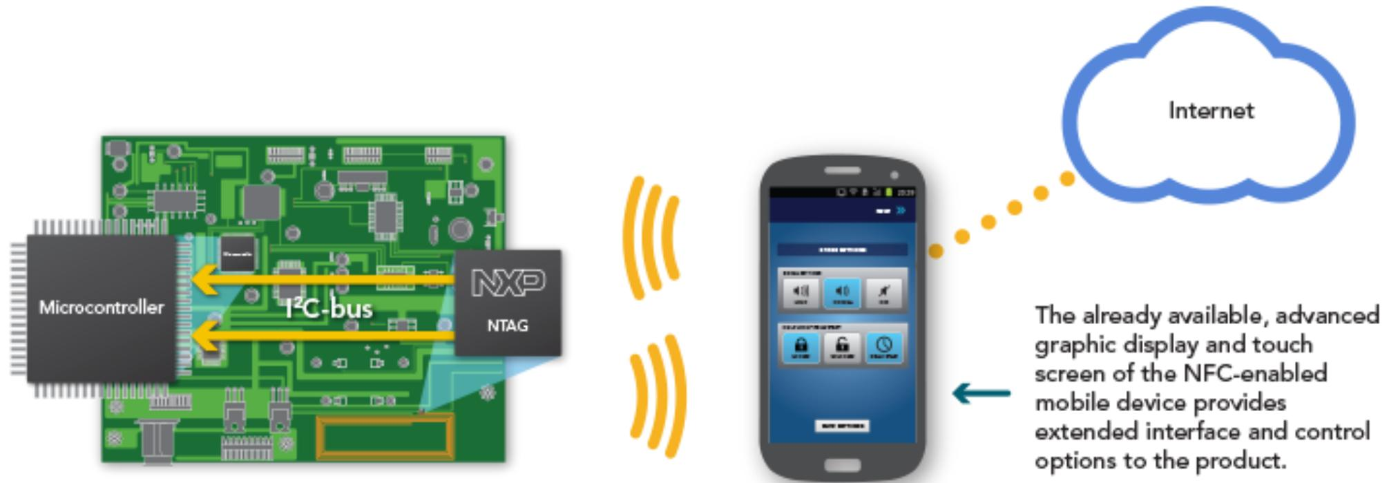
The NTAG I<sup>2</sup>C tag IC connects to the product's microcontroller via the I<sup>2</sup>C serial bus interface
